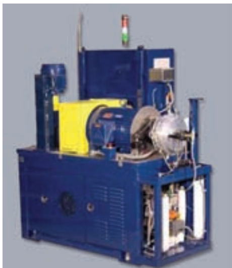
Figure 1. Full-scale clutch tests are conducted on test systems, such as the SAE #2 Friction Test Rig.
